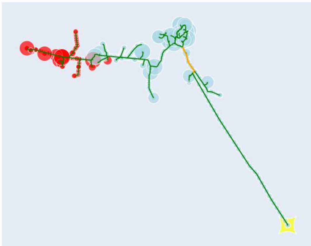
Figure 6.4. 127 simultaneous voltage violations at hour of the annual demand peak (20 July 2026, 12:00, 4.0 MW).
